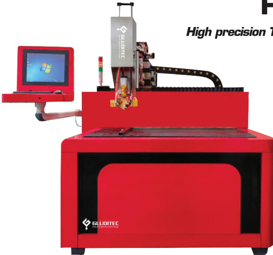
The GLUDITEC FAD-375P is engineered to deliver unparalleled precision in the metering and mixing of two-part polyurethane foam components. With advanced technology, this system ensures exact ratios of polyol and isocyanate, guaranteeing consistent and high-quality formulations for gasket adhesive applications.
