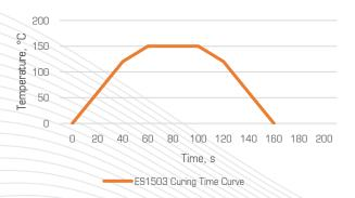
The product will obtain to higher bonding strength when higher curing temperature and longer cured time . the figure curve is the recommended curing temperature and heating rate, under the corresponding temperature ,components need the time when they achieve good bonding strength.
