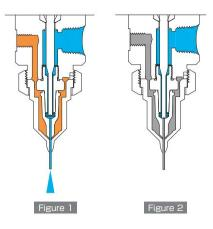
Input air pressure retracts the needle from the nozzle seat, allowing fluid to flow. At the same time, nozzle air flows around the nozzle and atomizes the fluid into fine droplets. (Figure 1) Once the cycle is completed, the spring returns the piston needle back to its position to shut off the fluid. (Figure 2).
