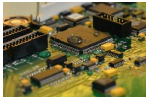
PCB with coating
